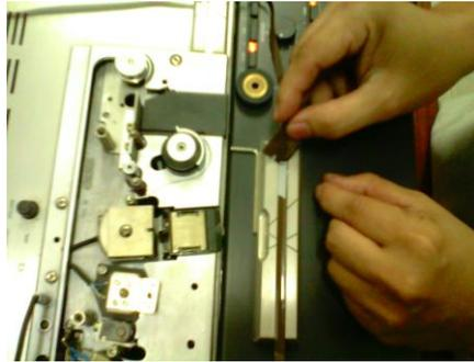
Figure 5 Slicing tape replacing
